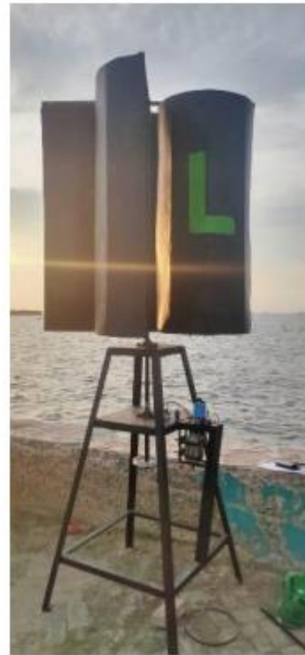
SET UP SAVONIUS WIND TURBINE 4 BLADES U TYPE
